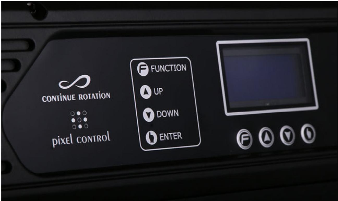
The spotlight has a display to show the set parameters and four buttons to adjust them.
